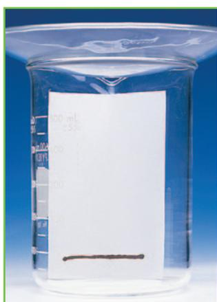
**(a)** Water-soluble ink is placed near the bottom of a piece of chromatography paper in shallow water.
