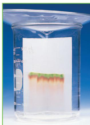
**(b)** The black ink separates into its component colors due to the different attraction between each component and water.
