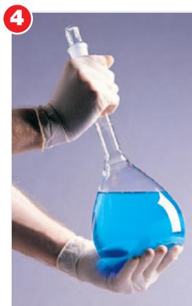
Put the stopper in the flask, and swirl the solution thoroughly.
