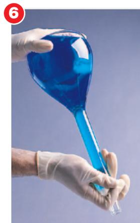
Restopper the flask, and invert it at least 10 times to ensure complete mixing.
