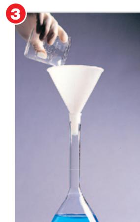
Rinse the weighing beaker with more solvent to remove all the solute, and pour the rinse into the flask. Add water until the volume of the solution nears the neck of the flask.
