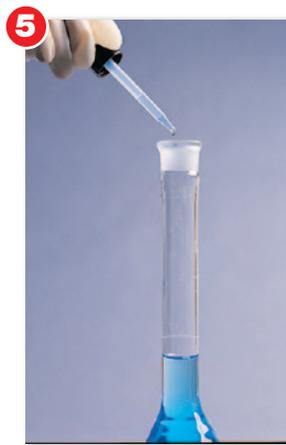
Carefully fill the flask to the 1.0-L mark with water.
