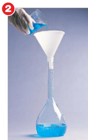
Add some solvent to the solute to dissolve it, and then pour it into a 1.0-L volumetric flask.
