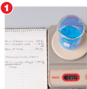
**1** Calculate the mass of  $\text{CuSO}_4 \cdot 5\text{H}_2\text{O}$  needed. Making this solution will require 0.5000 mol of  $\text{CuSO}_4 \cdot 5\text{H}_2\text{O}$  per kilogram of solvent (1000 g). This mass is calculated to be 124.9 g.
