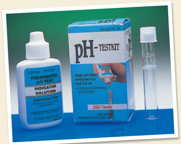
*The pH of your home's water supply can be easily monitored using a test kit, such as the one shown here.*
