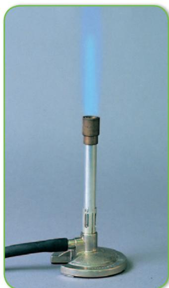
**(a)** In a Bunsen burner, methane combines with oxygen in the air to form carbon dioxide and water vapor.
