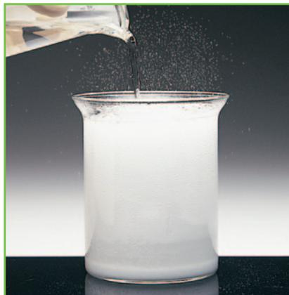
(a) The reaction of vinegar and baking soda is evidenced by the production of bubbles of carbon dioxide gas.
